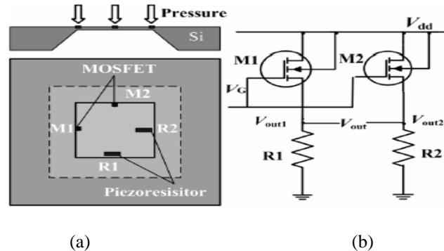
Figure 1. (a) Schematic of Novel MOSFET Pressure Sensor Including Two MOSFET and Two Resistors on the Membrane to Form a Wheatstone Bridge, (b) The MOSFET-Based Bridge Circuit, the Output Voltage is  $V_{out} = V_{out1} - V_{out2}$ , the Voltage Source is VDD
