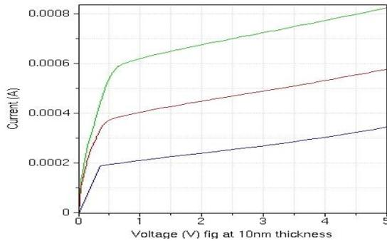
(a) Id-Vd Curve for Channel Thickness 10nm
