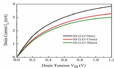
Figure2 ID vs.VDD Characteristics of Active MOSFET for Various Thickness of Oxide Layer [11].
