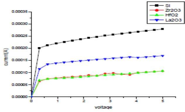
Figure 5. Id -Vd Curve at 2nm for Different Material
