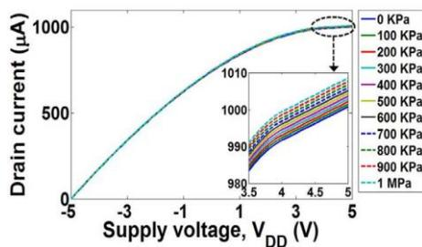
Figure 1 ID vs.VDD Characteristics of Active MOSFET for Various pressures [9].
