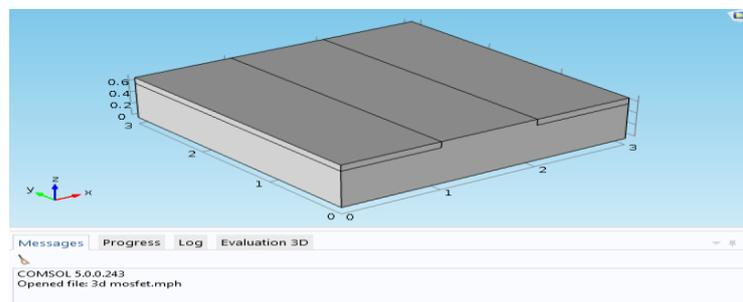
Figure 3. 3-Dimensional p Channel MOSFET of 3x3x.7 nm, Doped n-Region of Area 1x3nm Each Side with a p-channel Width of 1nm
