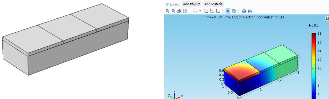
Figure 2. 3-D Model & Plot of Electron Concentration in the Model at Time=0 of p-channel MOSFET with Silicon Material
