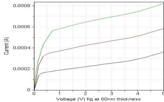
(b) Id-Vd Curve for Channel Thickness of 60nm
