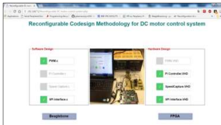
Figure 5. DC motor control web interface
