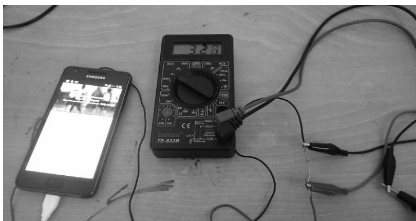
Figure 3. Experiment setup between multimeter and Samsung Galaxy S2 smartphone devices
