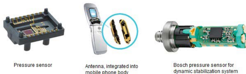
Figure 1. Examples of 3D-MID technology realization
