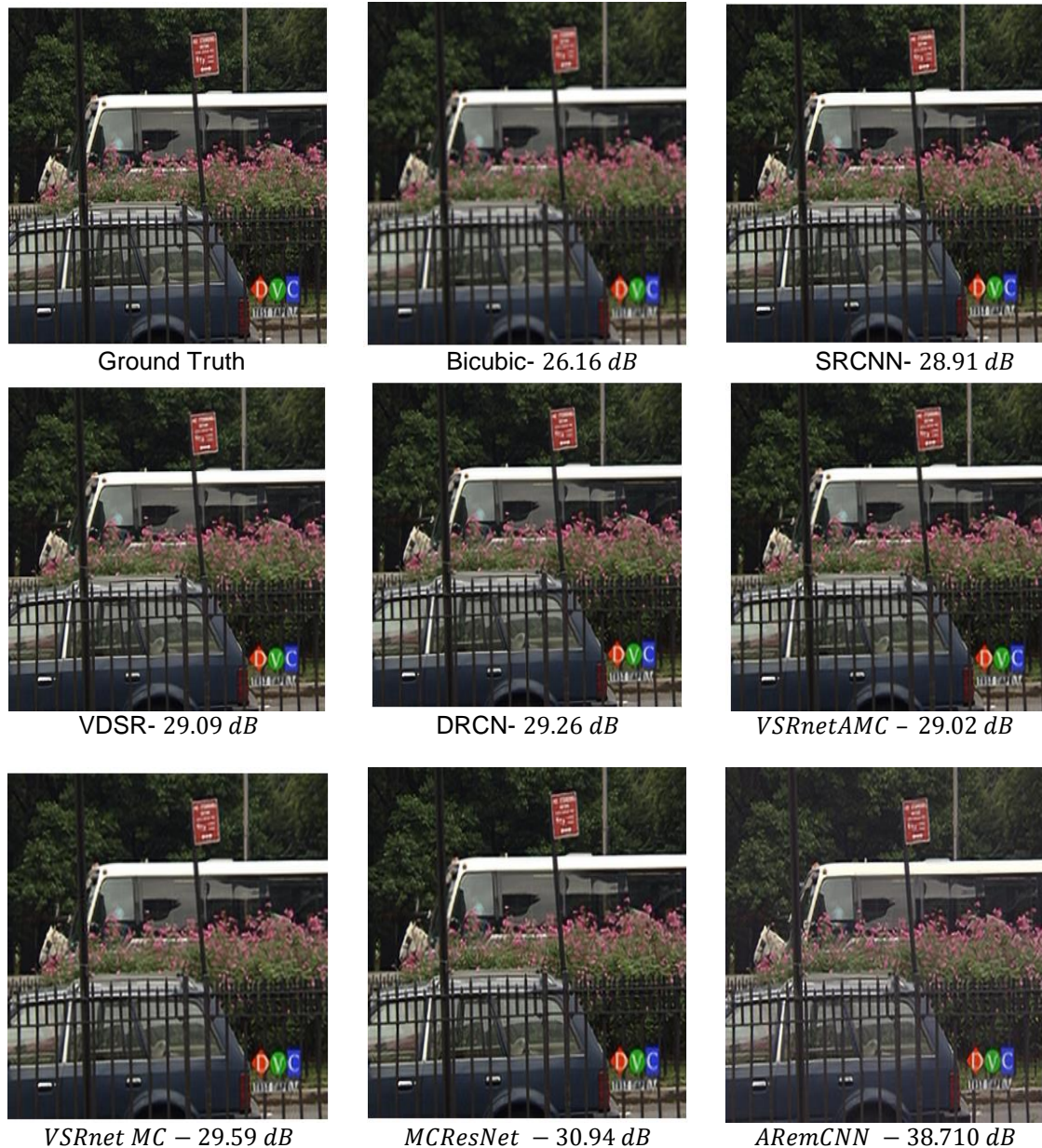
Figure 5. Bus video frame in the YUV21 dataset for scale factor 2 using different methods
