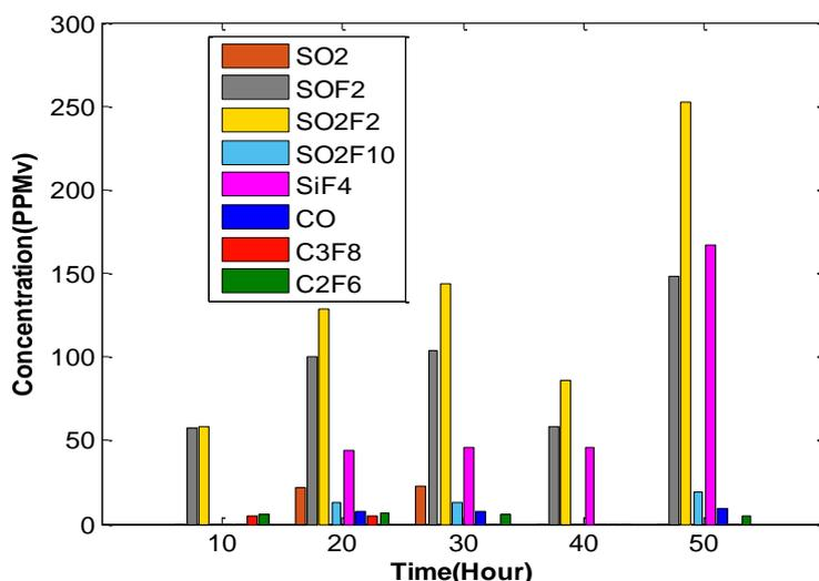
Figure 8b. Protrusion defect concentration of SF<sub>6</sub> decomposition product variation with time
