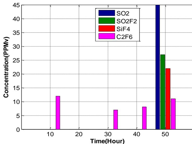
Figure 5b. Void defect concentration of  $\text{SF}_6$  decomposition product variation with time
