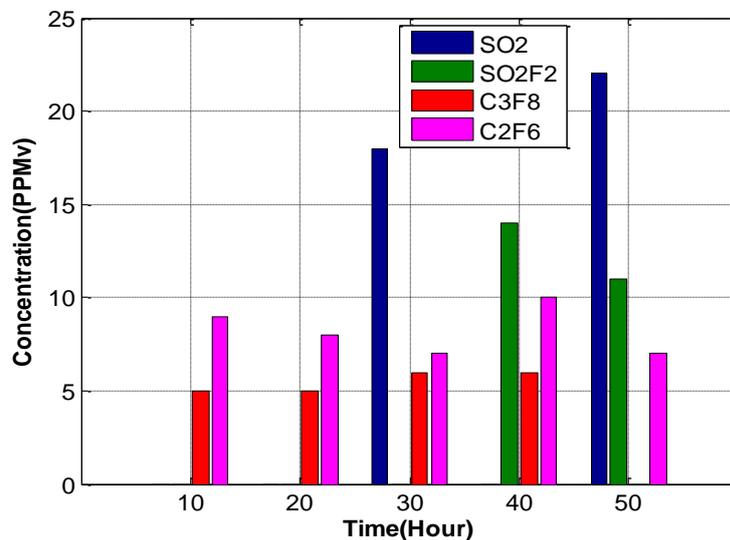
Figure 6b. Fixed defect concentration of SF<sub>6</sub> decomposition product variation with time
