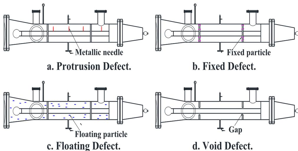
Figure 3. Designed four kinds of artificial defects
