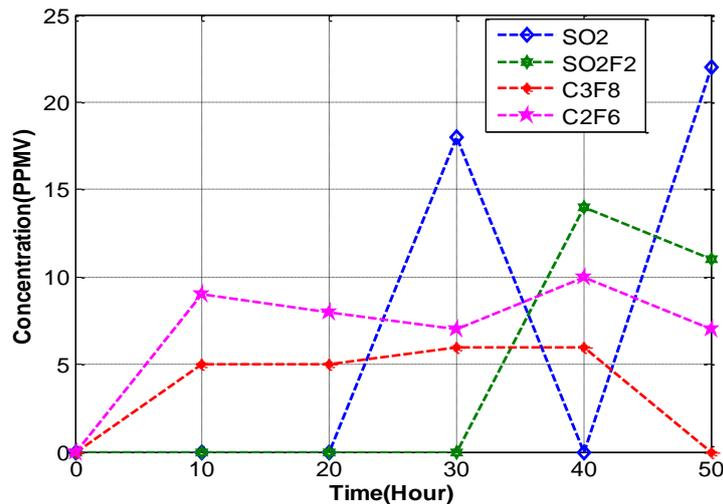
Figure 6a. Fixed defect concentration of SF<sub>6</sub> decomposition product variation with time
