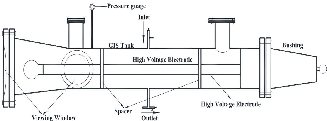
Figure 2a. SF<sub>6</sub> decomposition gas chamber
