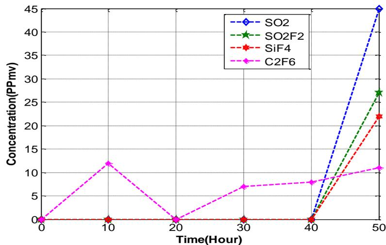
Figure 5a. Void defect concentration of  $\text{SF}_6$  decomposition product variation with time
