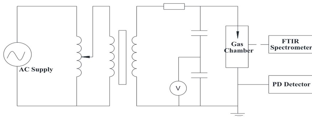
Figure 1a. SF<sub>6</sub> decomposition and detection system schematic diagram
