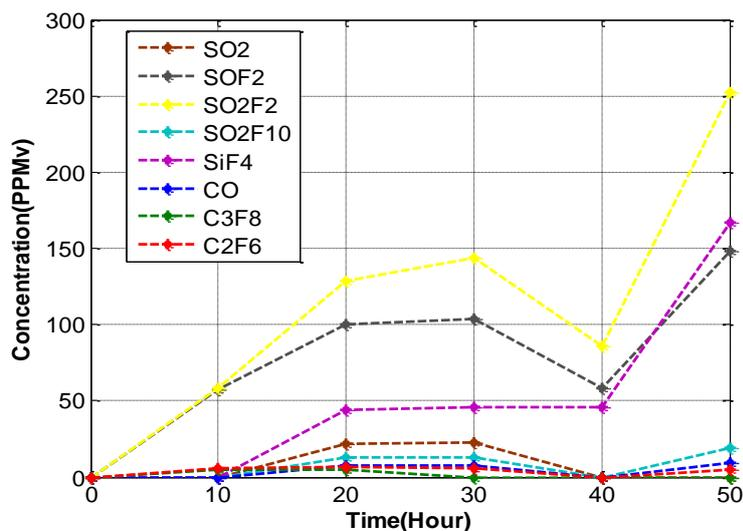
Figure 8a. Protrusion defect concentration of SF<sub>6</sub> decomposition product variation with time
