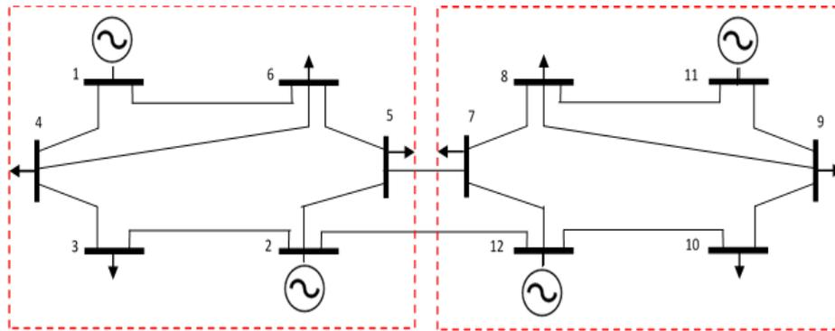
Figure 5. Single line diagram of 12-Bus System Model
