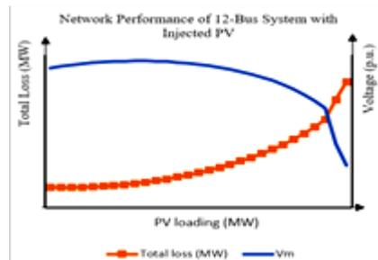
Figure 1. A network performance with injected non-optimized PV
