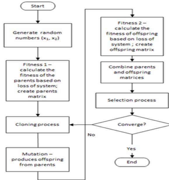
Figure 4. Flowchart of the IEP for optimal PV size and location
