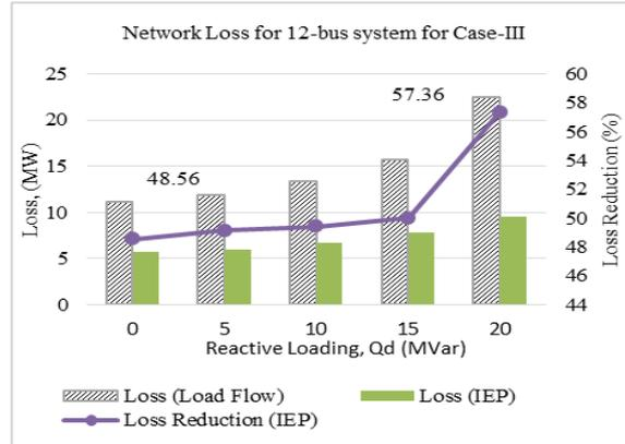
Figure 11. Effect of Optimal PV injection on three-reactively loaded bus of 12-bus system using IEP technique
