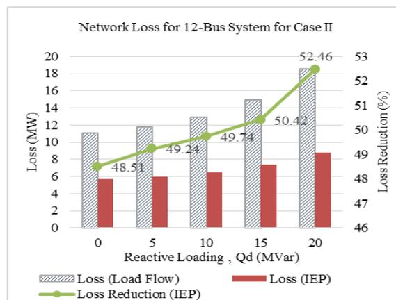
Figure 10. Effect of Optimal PV injection on two-reactively loaded bus of 12-bus system using IEP technique
