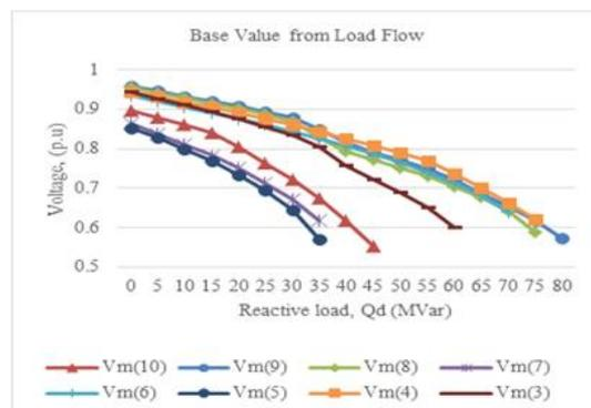
Figure 6. Base values of voltage from pre-optimized load flow of a 12-bus system
