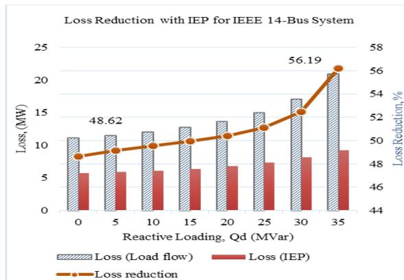
Figure 9. Effect of optimal PV injection on reactively loaded IEEE 14-bus system using IEP technique
