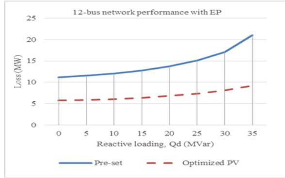
Figure 7. Network performance with increasing reactive load and PV injected
