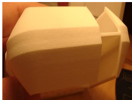
Figure 2. Good part surface by orange peel texture
