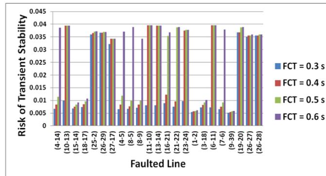
Figure 2. Risk of transient stability due to line fault at base case condition
