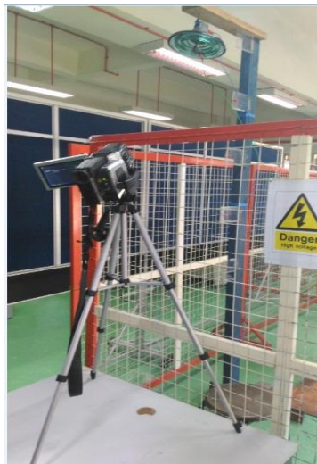
Figure 2. Experimental setup showing the thermal camera positioning
