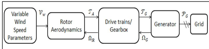
Figure 1. Variable speed wind turbine model
