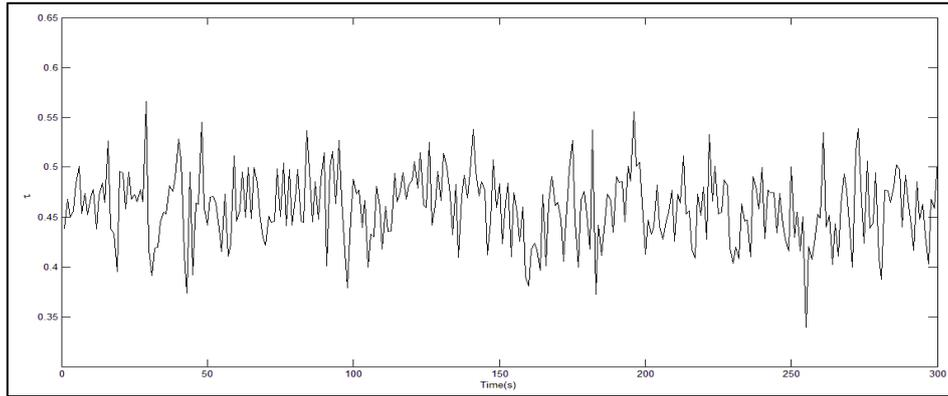
Figure 7. Aerodynamic torque variations observed due to wind speed variations
