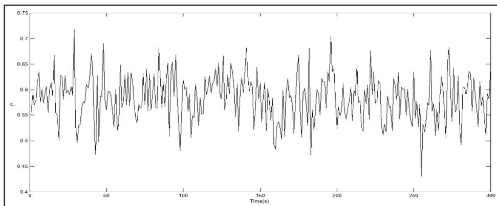
Figure 6. Aerodynamic power  $P$  delivered to main shaft considering variable wind speed
