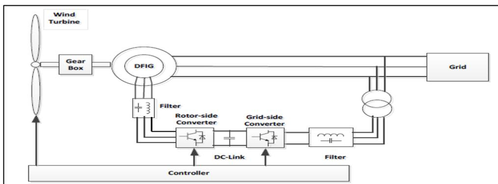
Figure 3. Grid connected wind turbine model for GDFIG and DFIG
