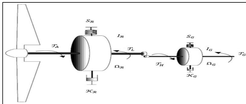
Figure 2. Wind turbine drive train dynamics
