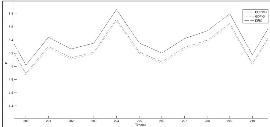
Figure 9. Performance comparison of power generated by DDPMG, GDFIG and DFIG under varying wind speed conditions at time interval of 200s to 210s
