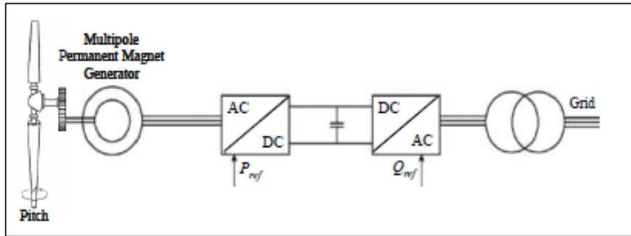
Figure 4. Grid connected wind turbine model of DDPMG
