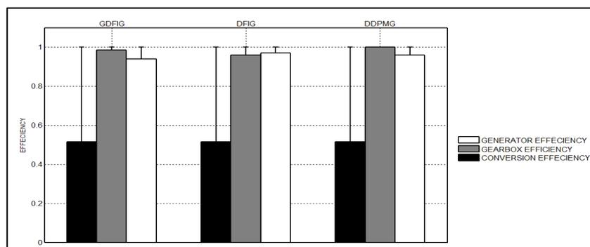
Figure 10. Conversion, gearbox and generator efficiency comparisons for GDFIG, DFIG and DDPMG
