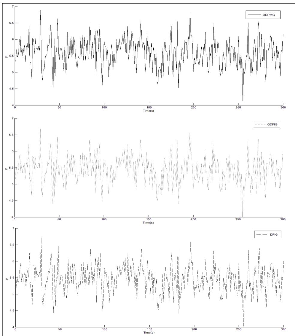
Figure 8. Performance comparison of power generated by DDPMG, GDFIG and DFIG under varying wind speed conditions
