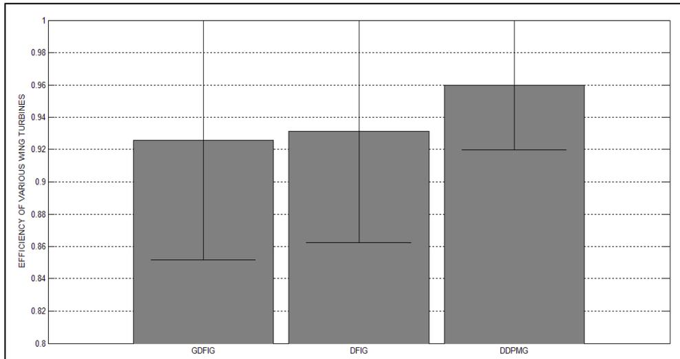
Figure 11. Wind energy conversion efficiency comparison for GDFIG, DFIG and DDPMG
