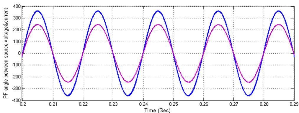
Figure 11. Power factor angle between source voltage and source current
