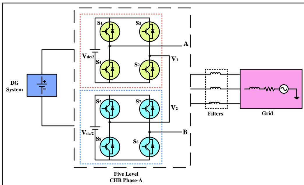
Figure 2. DG integration scheme to grid through 5-level inverter
