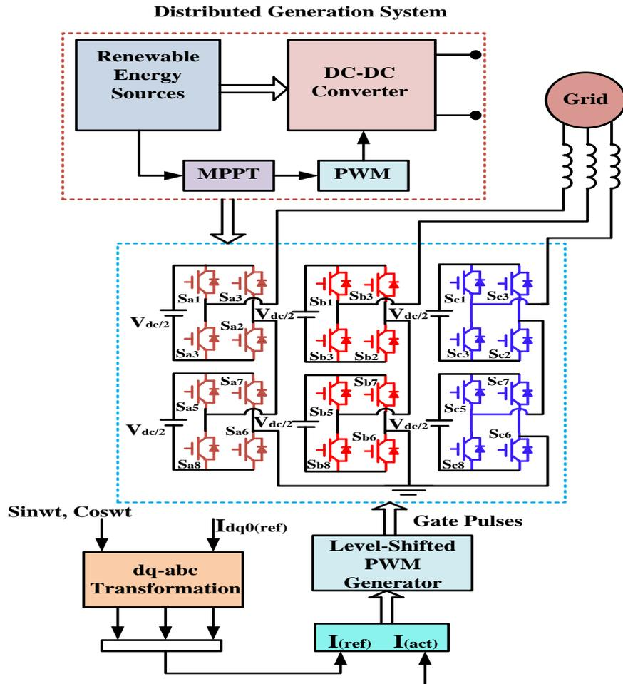
Figure 4. Complete picture of DG integration to grid through 5-level inverter with its control strategy
