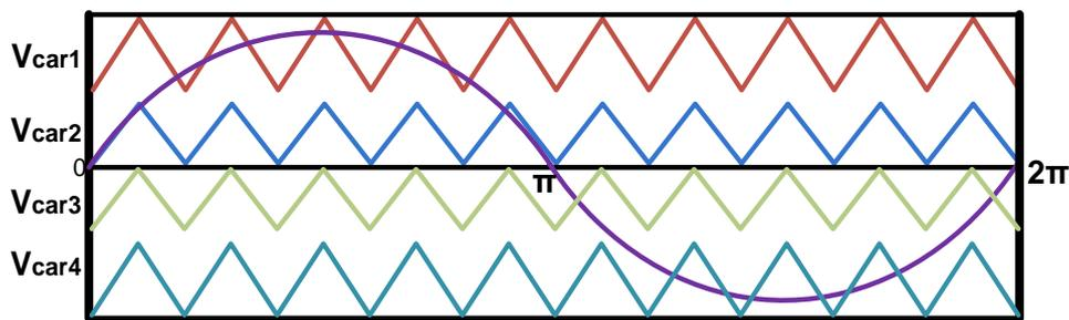
Figure 5. In-phase disposition PWM pattern
