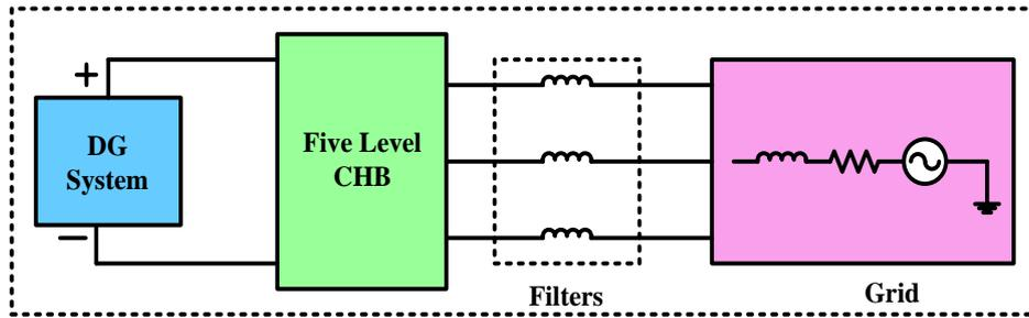
Figure 1. Schematic block diagram of DG integration to grid
