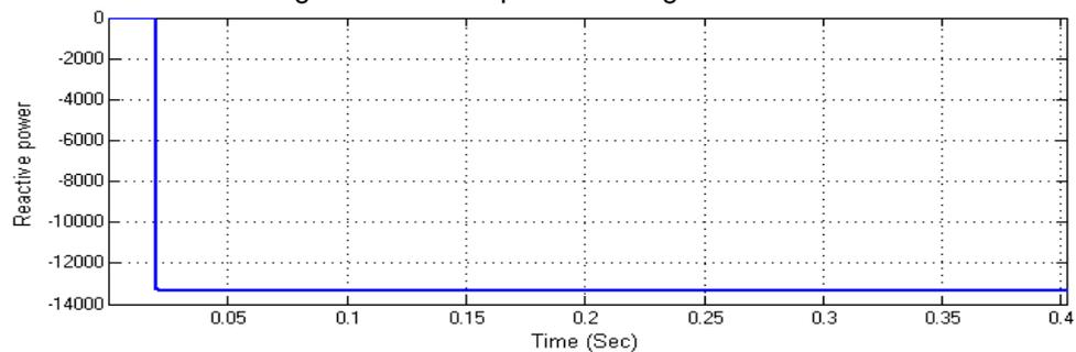
Figure 17. Reactive power fed to grid from DG
