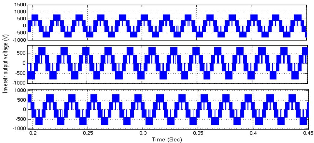
Figure 8. Three phase 5-level inverter output voltage
