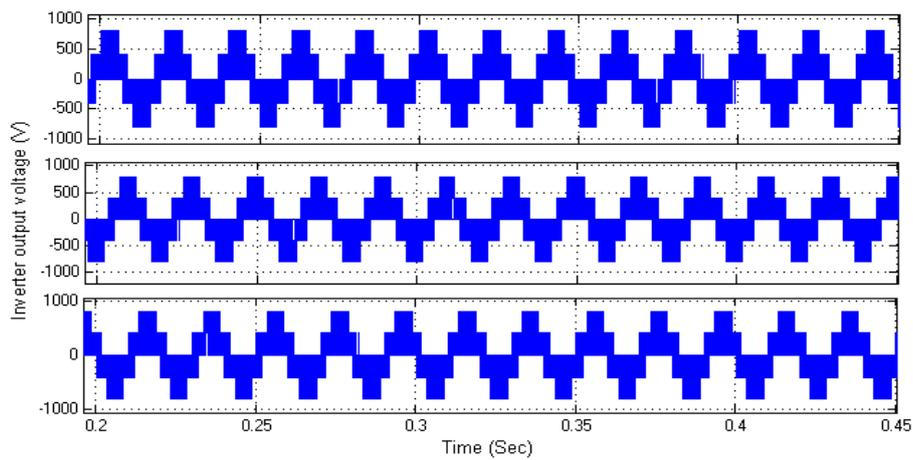
Figure 15. Three phase 5-level inverter output voltage
