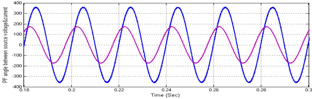
Figure 18. Power factor angle between source voltage and source current
