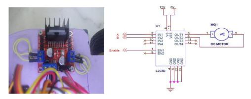
Figure 7. Driver L293 and schema
