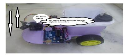
Figure 9. Final form of robot
