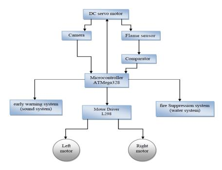
Figure 1. Block diagram
