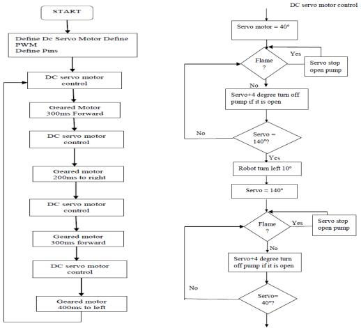
Figure 11. Fire tracking and suppression mobile robot algorithm
