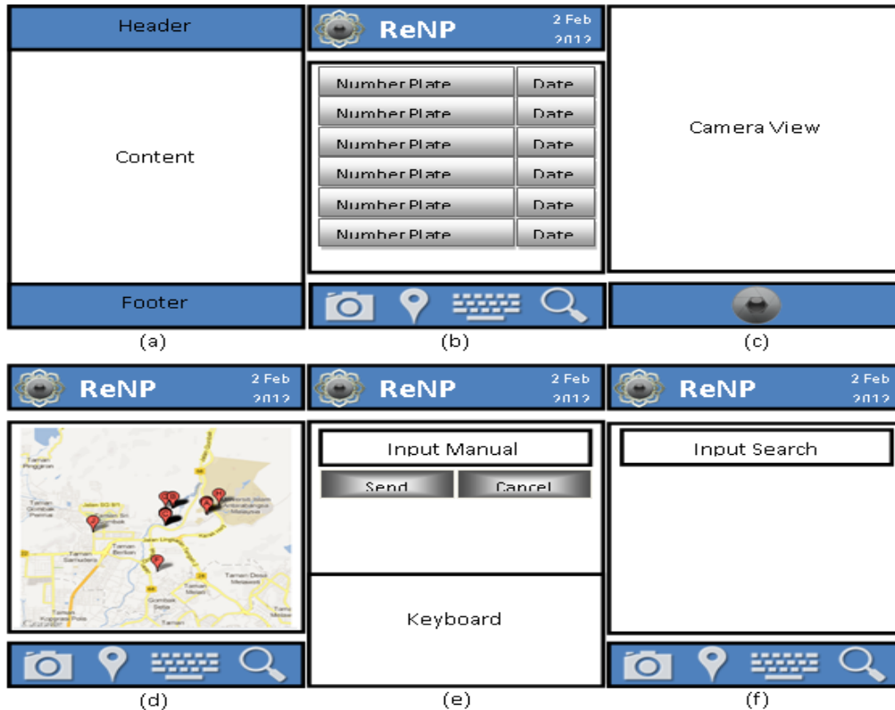
Figure 2. GUI, (a) Master layout of ANPR system, (b) Main page layout, (c) Capture page layout, (d) Map page layout, (e) Input manual page layout (f) Search page layout
