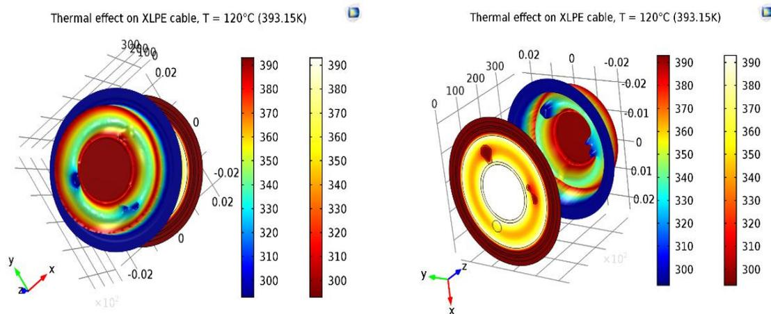
Figure 4c. Temperature distributions in XLPE cable at Maximum Overload Temperature:  $T = 120^{\circ}\text{C}$
