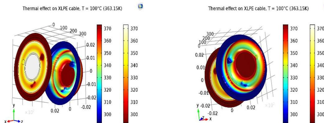
Figure 4b. Temperature Distributions in XLPE cable at Normal Operating Temperature: T= 100°C
