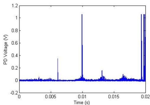
Figure 7a. Partial Discharge Activity before Heating Cycle at 120°C
