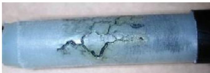
Figure 11. Damage of XLPE insulation due to accelerated ageing
