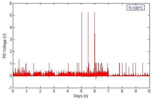
Figure 8a. PD voltage evolution during the heating cycles of 100°C: during the first ten days
