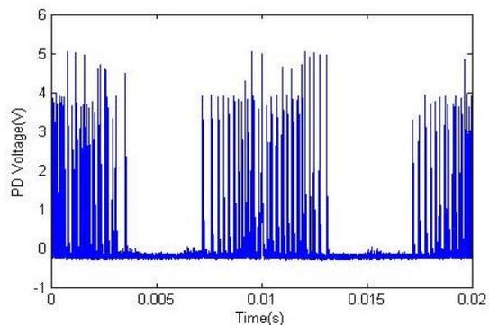
Figure 7b. Partial Discharge Activity after Heating Cycle at 120°C
