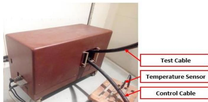
Figure 5. Load Current Transformer
