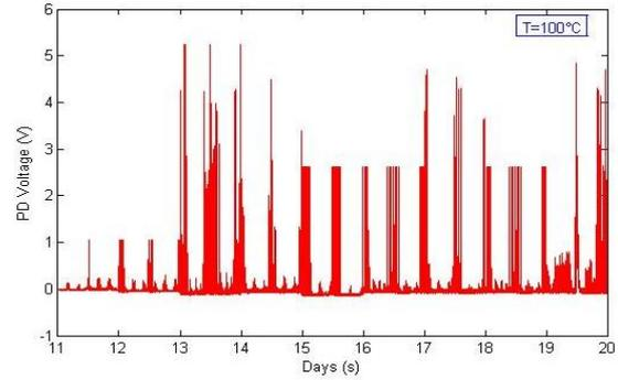
Figure 8b. Partial discharge activity after heating cycle at 120°C: during the last ten days
