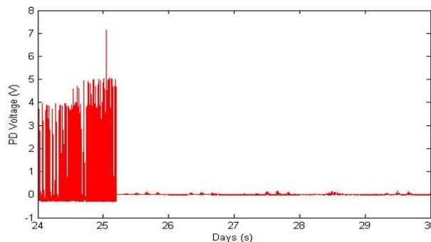
Figure 10. PD Voltage Evolution in the Sample with Artificial Cavity
