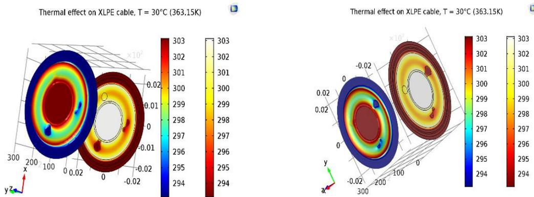
Figure 4a. Temperature Distributions in XLPE cable at Ambient Temperature: T= 30°C
