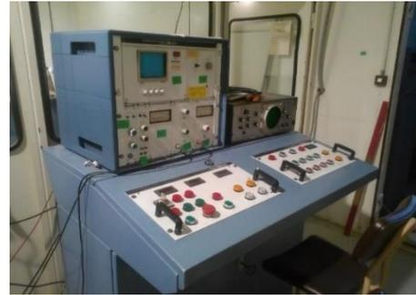
Figure 6b. Partial Discharge Detector
