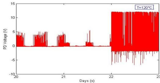
Figure 9. PD voltage evolution during the heating cycles of 120°C
