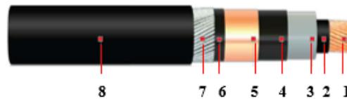
Figure 1. Physical Model of Single-Core 240 mm<sup>2</sup> XLPE Cable
