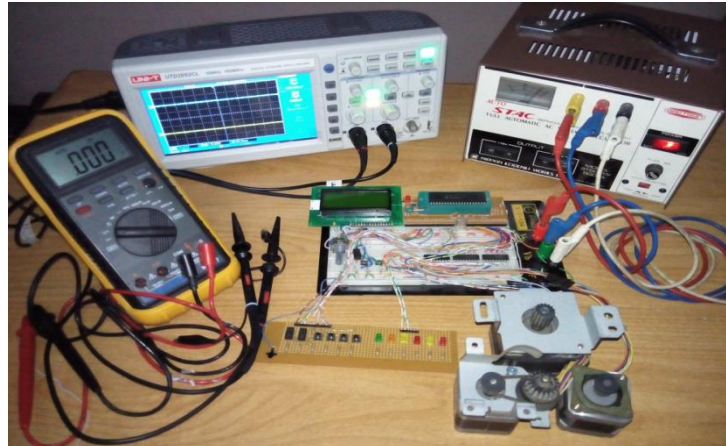
Figure 21. Photograph of the hardware setup connection of the multiple unipolar stepper motors position control system
