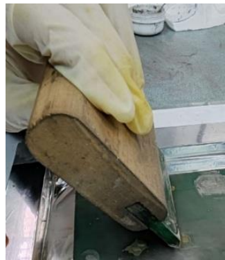
Figure 3. Stencils printing process on substrate
