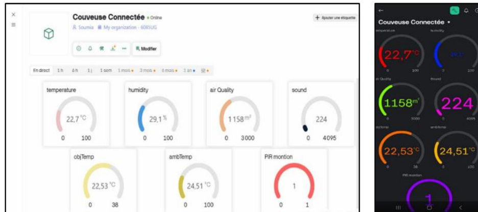
Figure 5. Real-time results on the Blynk dashboard and mobile application
