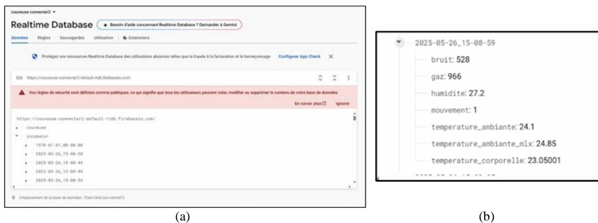
Figure 6. View of firebase real-time database (a) during live operation and (b) data store for a specific date
