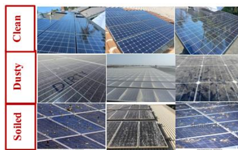
Figure 3. Clean, dusty and soiled samples of solar PV panel
