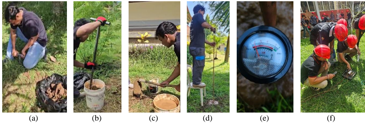
Figure 1. Samples processed, (a) boring and soil container, (b) soil engineering, (c) backfilling, (d) electrode, (e) pH level testing, and (f) Grounding resistance testing
