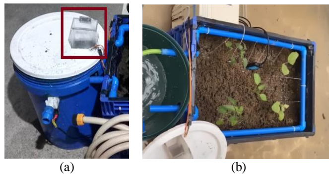
Figure 3. The physical configuration (a) fertilizer dispenser subsystem and (b) irrigation system setup integrated into the planting bed
