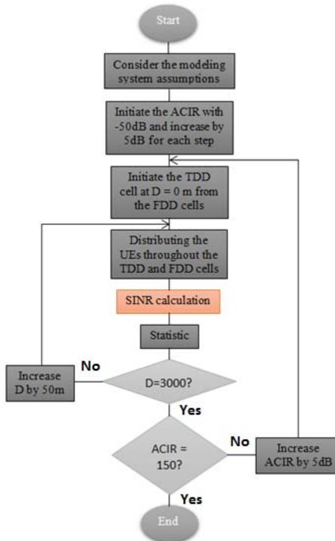
Figure 3. The general simulation algorithm
