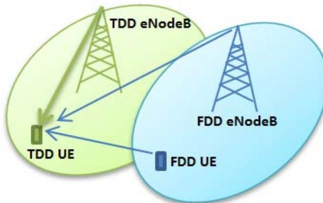
Figure 2. The interference of the TDD uplink and downlink at the FDD downlink
