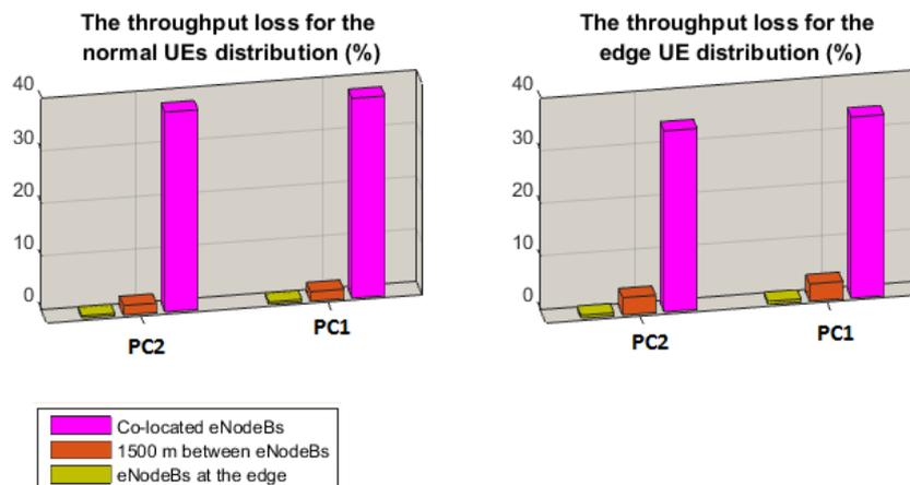
Figure 8. The expected throughput loss for the TDD downlink case
