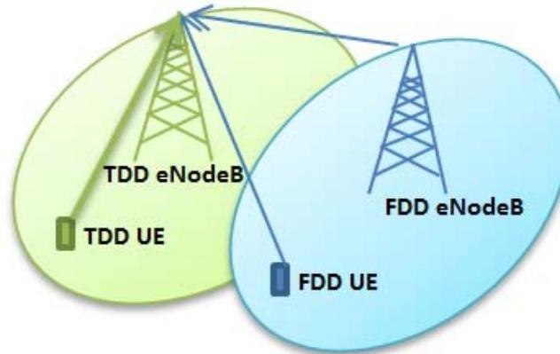
Figure 1. The interference of the TDD uplink and downlink at the FDD uplink
