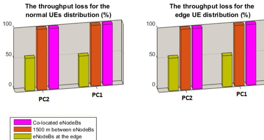
Figure 7. The expected throughput loss for the TDD uplink case
