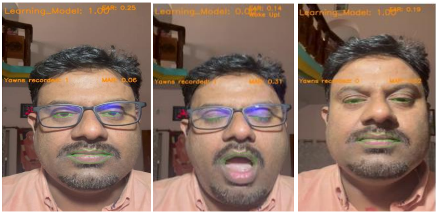
Figure 4. Demonstrates real-time testing of the proposed drowsiness detection model
