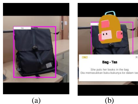
Figure 7. Result of integration: (a) object detection with YOLO and (b) augmented reality integration
