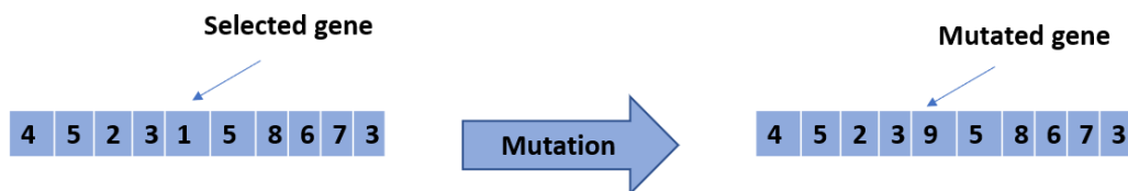
Figure 5. The mutation mechanism
