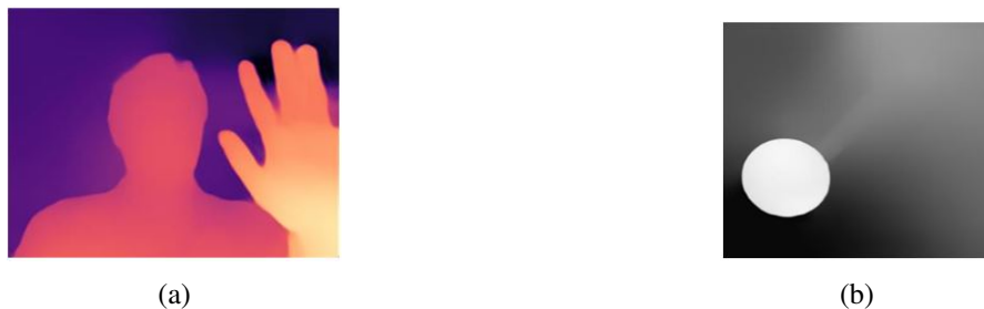
Figure 3. Depth map is visualized with colors that indicate the relative distances of the objects (a) MiDaS small algorithm example and (b) proposed image processing for monocular architecture.
