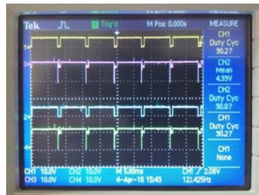
Figure 18d. PWM signals and motors terminal voltage at duty cycle 90% and 90% (speed n_1 = n_2 )
