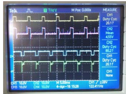
Figure 18b. PWM signals and motors terminal voltage at duty cycle 20% and 80% (speed n_1 < n_2 )
