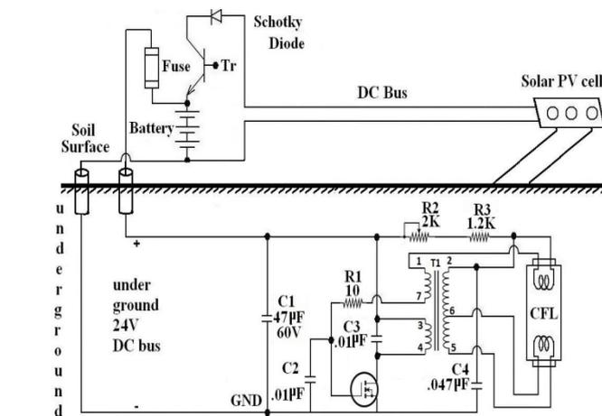
Figure 2. Fly-back inverter for operating CFL using MOSFET
