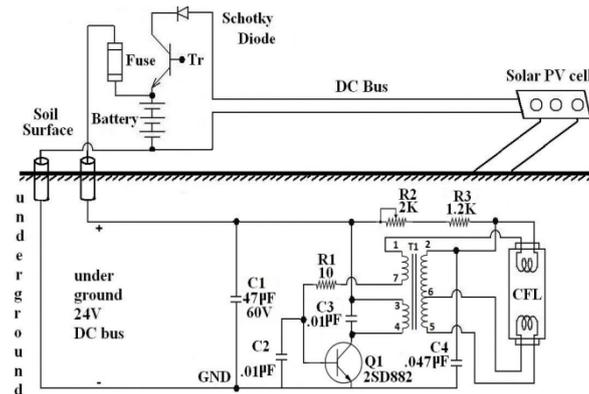
Figure 3. Fly-back inverter operating using BJT
