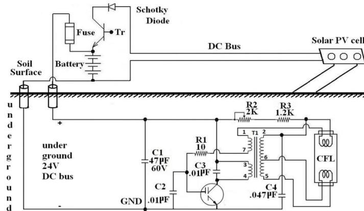
Figure 1. Fly-back inverter for operating CFL using MCT
