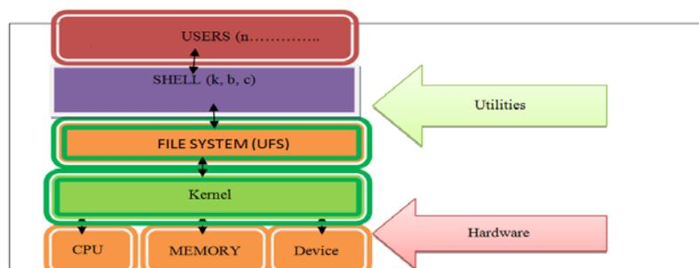
Figure 1. Internal Structure of RTOS
