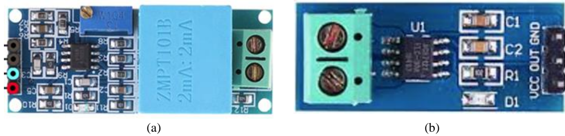
Figure 2. Sensors used (a) voltage sensor and (b) current sensor
