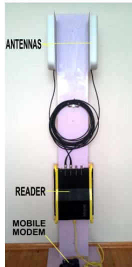
Figure 7. Hardware part of the web-based RFID personnel monitoring system
