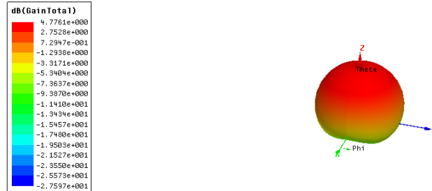
Figure 11. 3D polar plot of total Gain of PRMPA with an ‘inverted SHA’ shaped DGS
