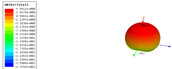
Figure 9. 3D Polar Plot of Total Directivity of PRMPA with an ‘inverted SHA’ Shaped DGS
