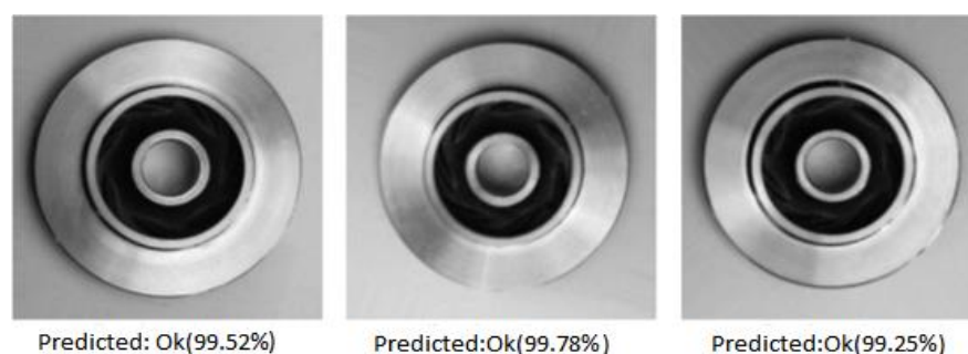
Figure 3. Shows the Identification of casting surface defects (ok)
