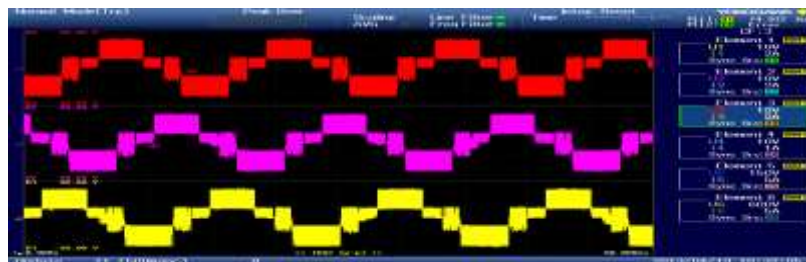
Figure 13. Experimental Output Voltage with APODPWM Strategy for R-Load
