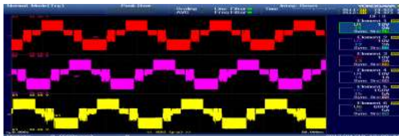
Figure 17. Experimental Output Voltage with PSPWM Strategy for R-Load
