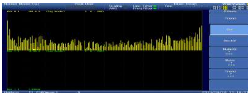
Figure 20. FFT Plot with VFPWM Strategy for R-Load
