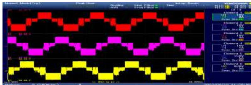
Figure 9. Experimental Output Voltage with PDPWM Strategy for R-Load
