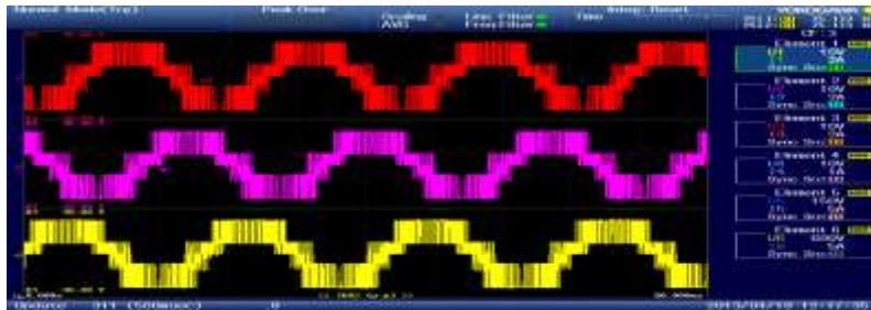
Figure 15. Experimental Output Voltage with COPWM Strategy for R-Load
