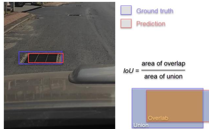
Figure 11. An example of a prediction and ground truth bounding box. The ground truth box is represented in blue, while the prediction bounding box is depicted in red
