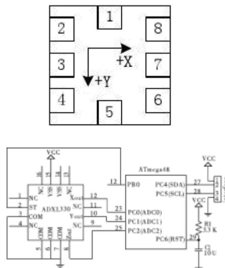
Figure 1. The Circuit Principle Diagram of Sensor Network Node
