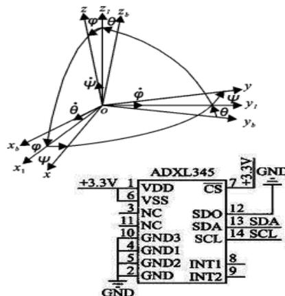
Figure 3. ADXL345 Digital Three Axis Accelerometer Structure Diagram
