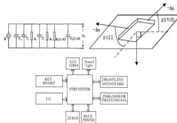
Figure 2. The Hardware Connection Diagram
