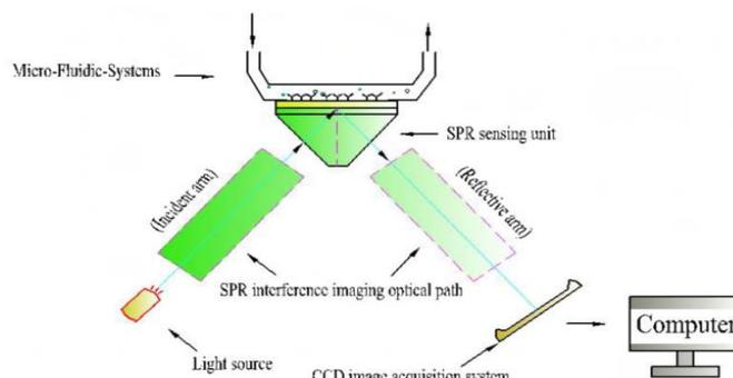
Figure 1. SPR Imaging Detection of Biomolecular Interaction Experiment Device
