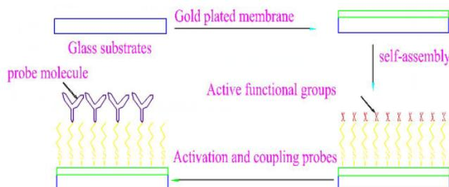
Figure 3. SPR Sensor Chips Preparation Process Schematic Diagram
