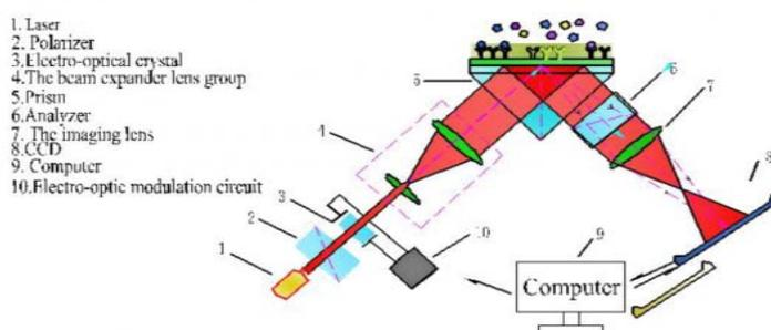
Figure 2. SPR Interference Imaging Light Path
