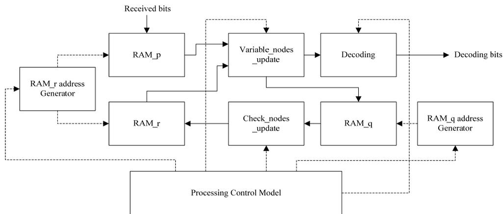
Figure 4. The Structure of (2560, 1024) QC-LDPC Decoder
