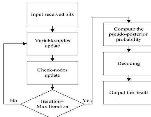
Figure 3. The Procedure of (2560, 1024) QC-LDPC Decoder
