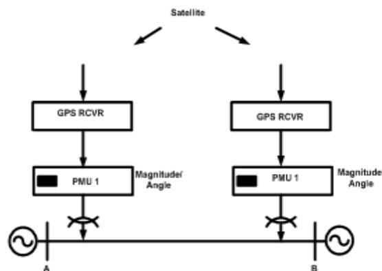
Figure 3. PMU provision at sending end and receiving end
