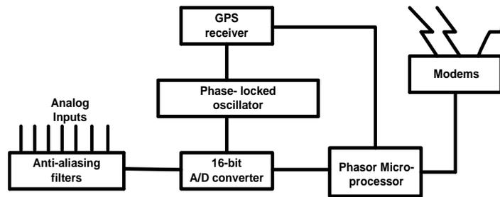
Figure 1. Functional block diagram of PMU
