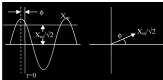
Figure 2. Waveform and phasor representation
