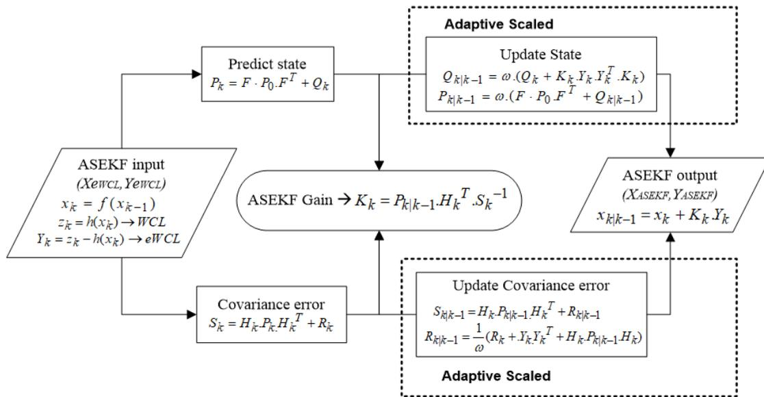
Figure 3. The main calculation processes of ASEKF algorithm
