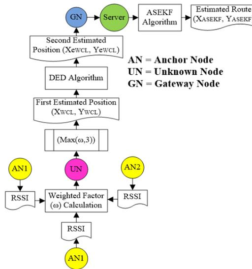
Figure 1. RSSI based adaptive tracking system methodology
