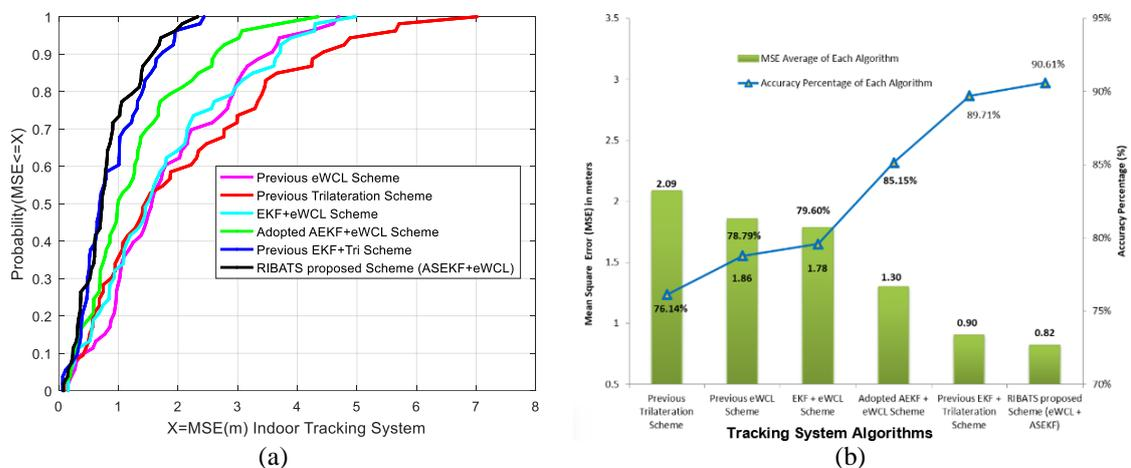
Figure 5. These figures are (a) CDF graph of RSSI-based adaptive tracking system and (b) Pareto chart of RSSI-based adaptive tracking system
