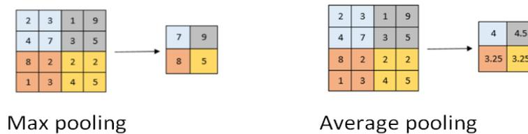
Figure 6. Max and average pooling operation
