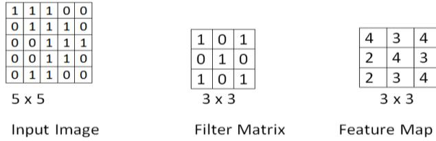
Figure 4. Convolution operation of input image with filter
