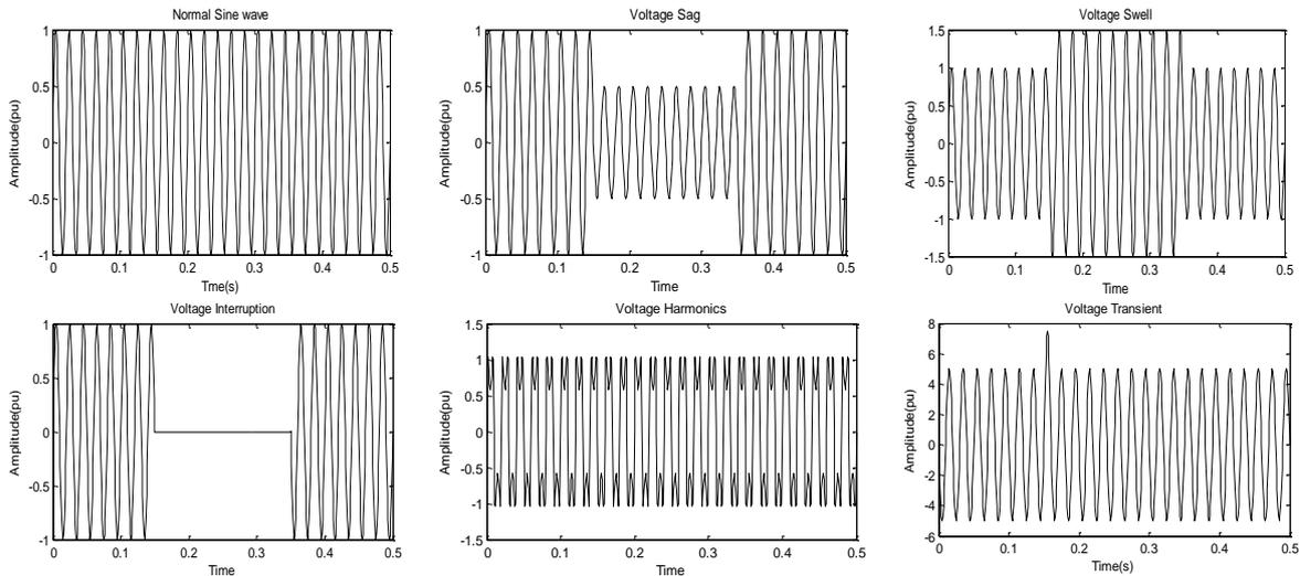
Figure 10. Samples of PQ problems generated in MATLAB
