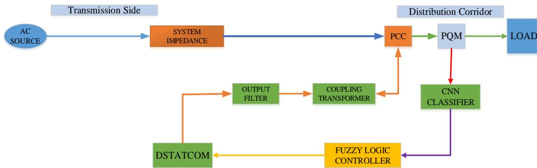
Figure 8. Complete block diagram of CNN – FLC - DSTATCOM approach
