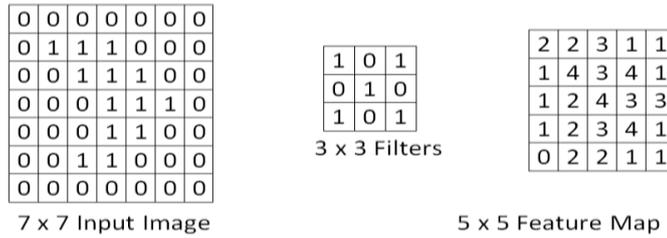
Figure 5. Convolution operation using padding technique
