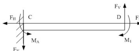
Figure 7. Photo of force analysis about single cantilever
