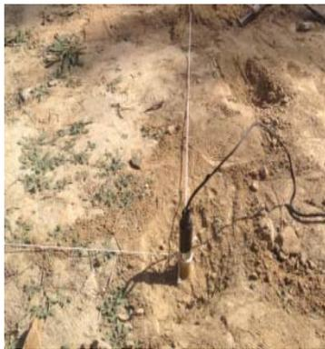
Figure 9. Method of the MEMS acoustic vector sensor buried
