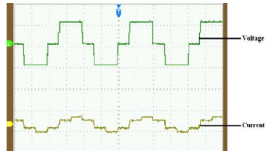
Figure 7. Line voltage and line current waveforms for star connected load
