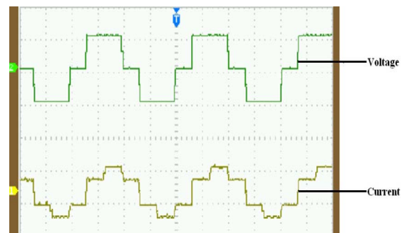
Figure 9. Line voltage & current for delta connected
