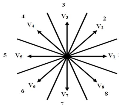
Figure 2. Definition of SRM motor voltage vectors for DTC
