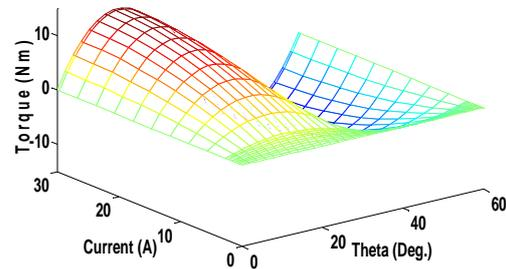
Figure 4(b). Mesh plot of Torque-current-angle
