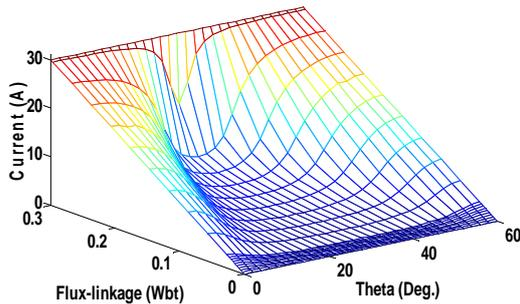
Figure 4(a). Mesh plot of flux-current-angle
