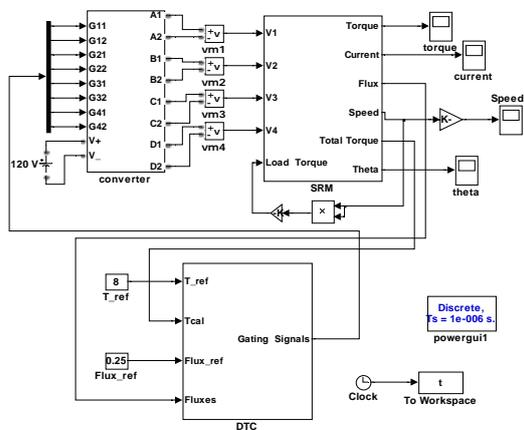
Figure 3(a). Simulation model of DTC based drive
