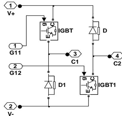
Figure 5(b). One leg of the converter
