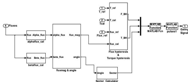
Figure 6. Torque computation block
