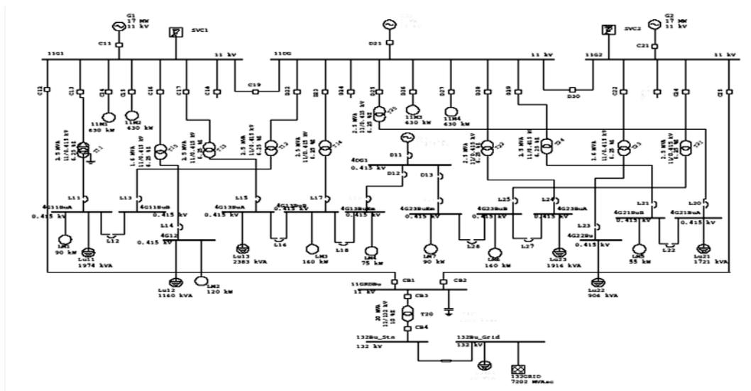
Figure 1. Network Diagram for System Study
