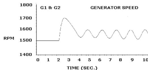
Figure 2. Generator speed (RPM) vs. Time (sec.)
