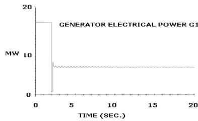
Figure 5. Generator active power (MW) vs. Time (sec.)
