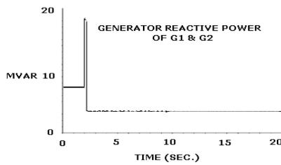
Figure 6. Generator reactive power (MVAR) vs. Time (sec.)
