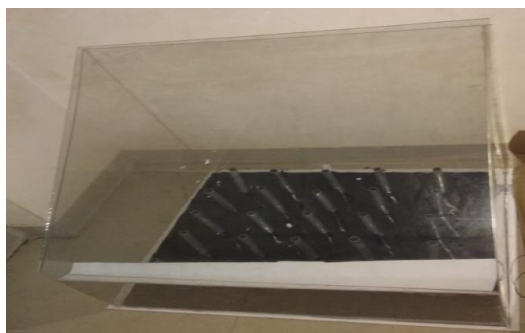
Figure 5. Acrylic box and L shaped water collector with glass cover
