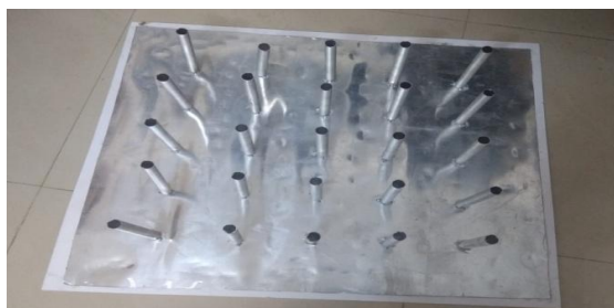
Figure 4. Aluminium fins as heat storage material
