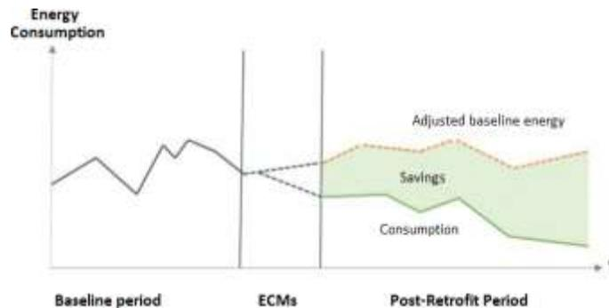
Figure 1. M&V conceptual structure
