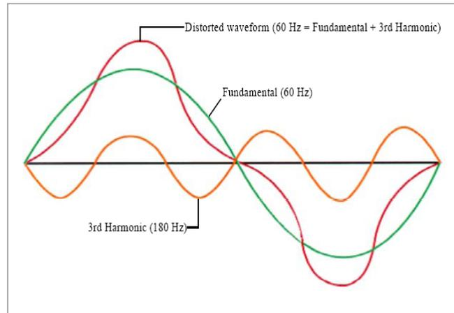
Figure 2. Fundamental and 3<sup>rd</sup> Harmonics
