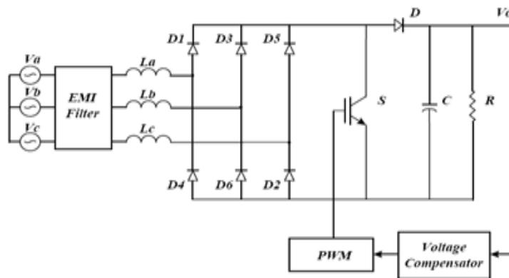
Figure 3. A Single-switch Three-phase Boost Rectifier
