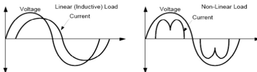
Figure 1. Current and Voltage Waveforms for Non-linear Load
