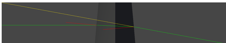
Figure 4. The guidelines, for instance, in the case of the principal ray at the top of the lens, are as follows: the green lines represent the ray’s trajectory, the red lines correspond to the normals at the points where the ray collided, and the yellow line is used to project the resulting ray
