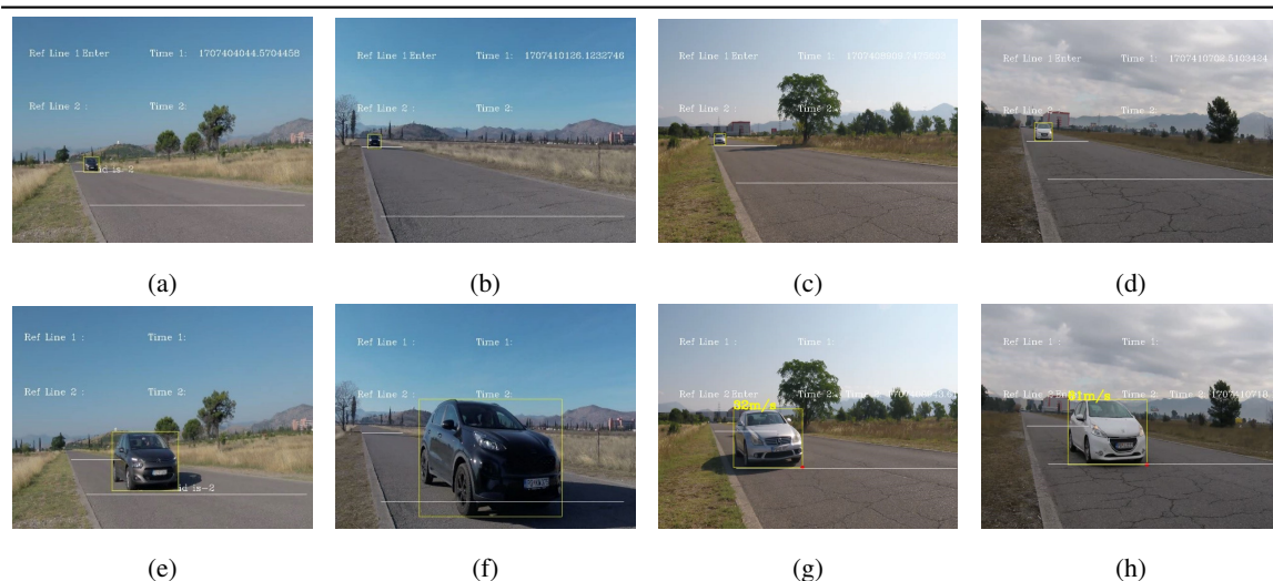
Figure 3. Simulation results of vehicle monitoring: (a)-(h) speed measurement and reference line crossing using the proposed approach
